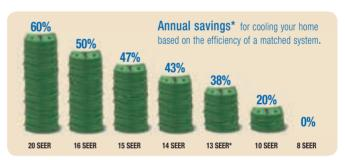
\*Minimum efficiency established by the Department of Energy. The majority of systems installed prior to 2006 are 10 SEER or lower. Potential energy savings may vary depending on your lifestyle, system settings, equipment maintenance, local climate, home construction and installation of equipment and duct system.
